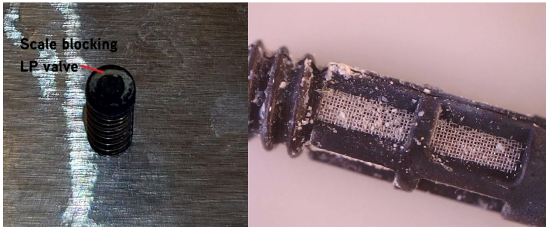
Scale blocking full seal of the LP nozzle valve + clogged nozzle filter
